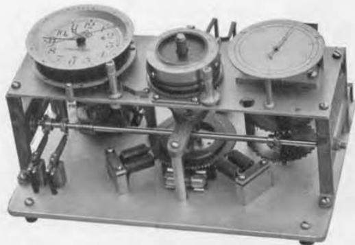
TYPE 511 Syncro-Clock with special micro-dial which permits time-interval comparisons to be made within 0.01 second
