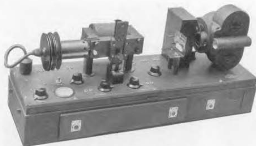
Recording Oscillograph Used in oil-locating surveys
