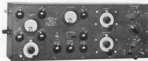
Antenna-Measuring Equipment. A portable unit for studying antenna characteristics
