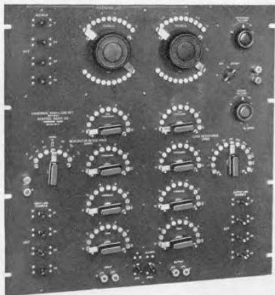
Universal Gain-Loss Set for determining transmission characteristics of circuits and component parts
