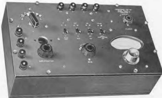
TYPE 355 Transformer Test Set. An early ex- ample of test apparatus
