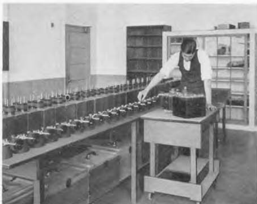
Individual calibration of TYPE 358 Wavemeters
